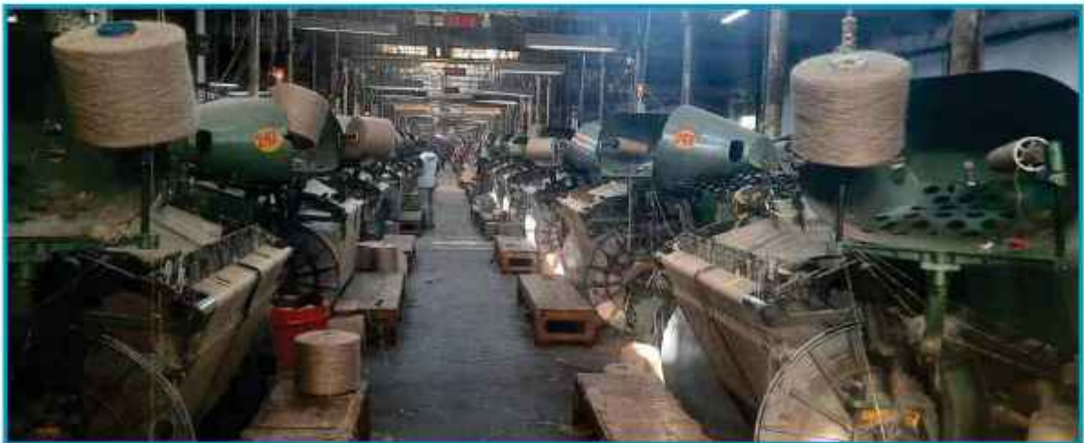
54A Jute Circular Looms in Ludlow Jute and Specialities Ltd.
