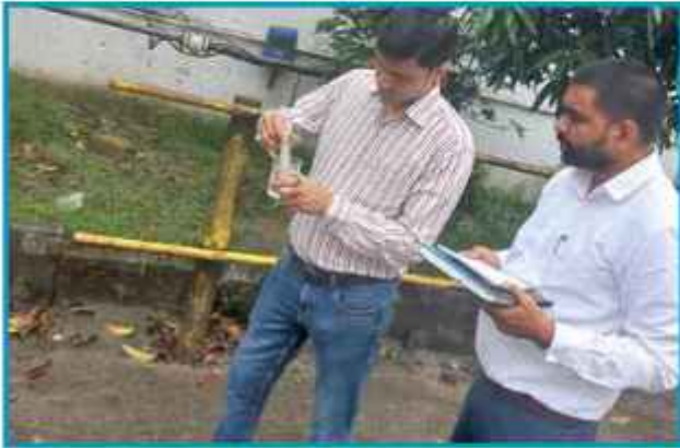
Checking of TDS of Ground Water during Audit
